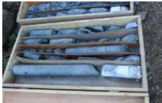
Fig. III-3: Core sampling for RQD parameter calculation
